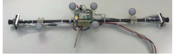
Figure 6. The stereo rig used during the experiments.
